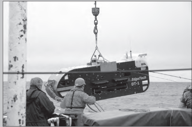
Deployment + retrieval of a sidescan sonar. The device transmits direct images of the seabed to the scientific crew on board the ship. 2006 marine geological investigations, west coast of Greenland. Photo: NunaOil
