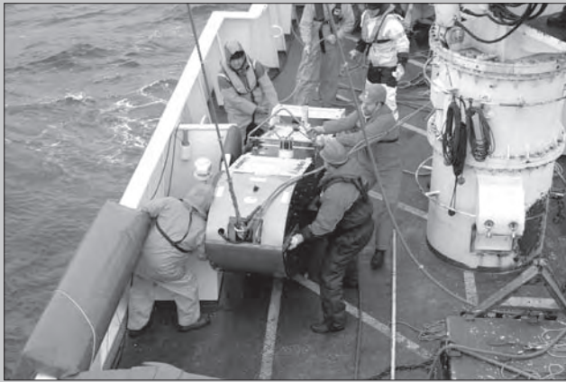
Deployment + retrieval of a sidescan sonar. The device transmits direct images of the seabed to the scientific crew on board the ship. 2006 marine geological investigations, west coast of Greenland. Photo: NunaOil
